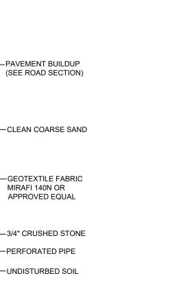
TYP. PERFORATED UNDERDRAIN TRENCH SECTION NOT TO SCALE
